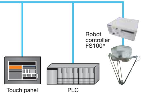
\*: You can also use an EXU-001 Rack Expansion Interface Unit to connect to the bus. Contact your Yaskawa representative for information on connecting robot controllers.
