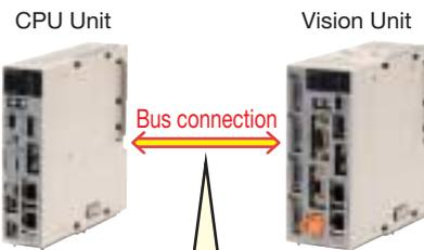
Connect the CPU Unit and the Vision Unit directly with the high-speed bus for simple system design.
